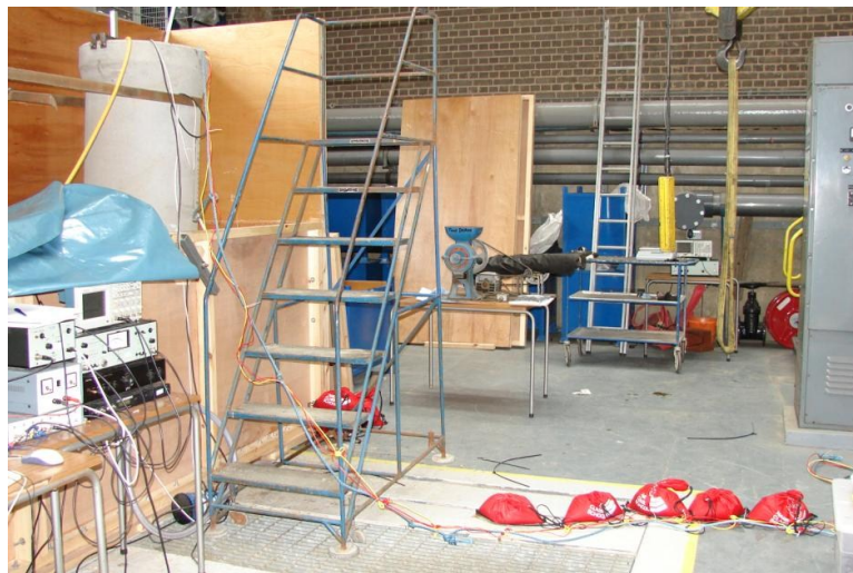
Figure 4. Sandbags are prepared for the insertion into the siphon.
